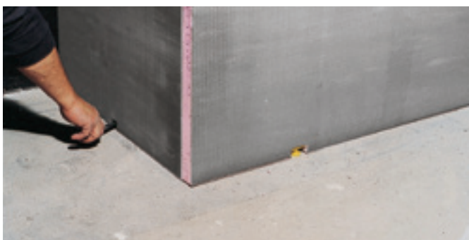
Practical levelling foot made of hard plastic. Can be easily set to precisely the required height (up to approx. 10 cm) using a 17 mm open-end wrench.
