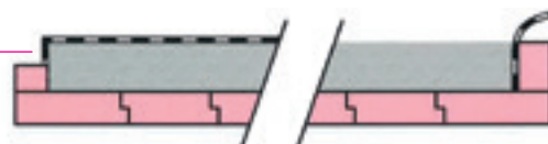
Foundation formwork with horizontal seal
